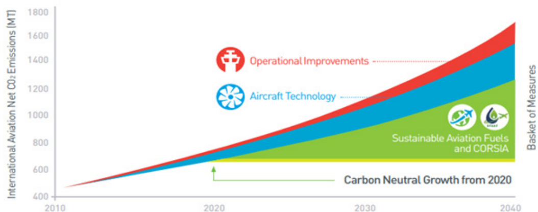
Figure 1: The contribution of different measures for reducing net CO 2 emissions from international aviation 7
